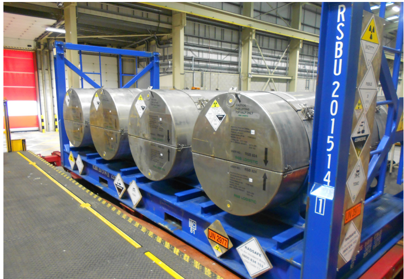
Overpacks containing enriched UF_6 cylinders (Image courtesy Urenco)
